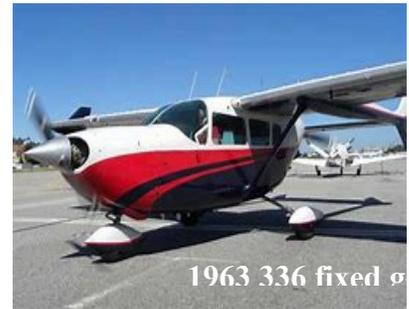
In 1963 Cessna introduced the 336 fixed-gear Skymaster with a 0.187 windshield. Common practice to avoid stress cracking, brittle windshields were secured floating in a soft felt surround. Like early plastics, early adhesives would also predictably fail over time.
