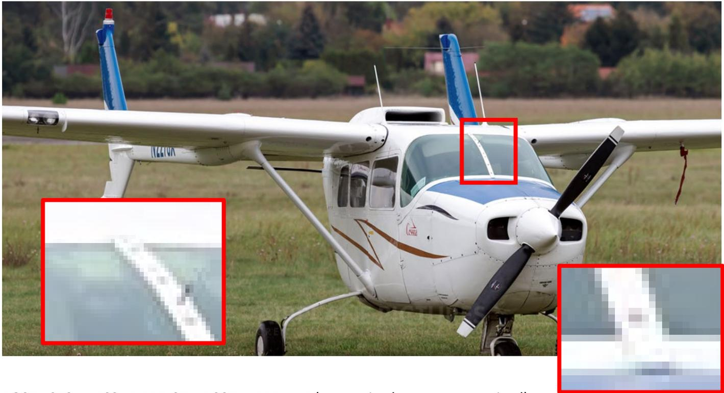
POST 1973 ***PRESSURIZED-STYLE*** 337 AIRFRAME (pressurized or non-pressurized)
