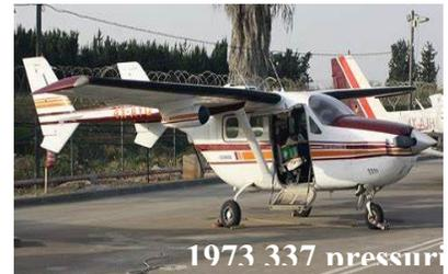
Instead of manufacturing two 337 airframe styles, all Skymasters manufactured after 1973 adopted the same 'pressurized' airframe design, pressurized or otherwise.
