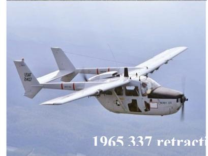
In 1965 Cessna introduced the 337 (retractable) with a thicker 0.250 windshield secured in the same manner as the 336.
