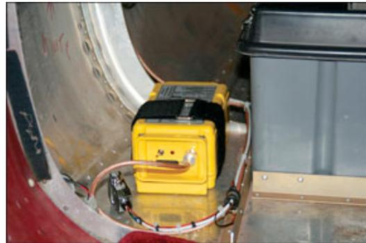
**Just looking at this Artex ME406 makes the install look trivial. The hidden cost is in wiring to the remote switch and optional GPS connection.**
