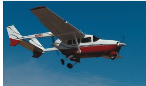
That's a 1965 337 wearing a modern paint scheme. It also has the finicky hydraulic landing gear used on the Cessna 210 Centurion, later upgraded to electro-hydraulic.
