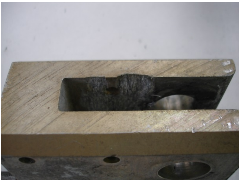
Cessna 200 series spar cap block attachment fittings corrosion damage
