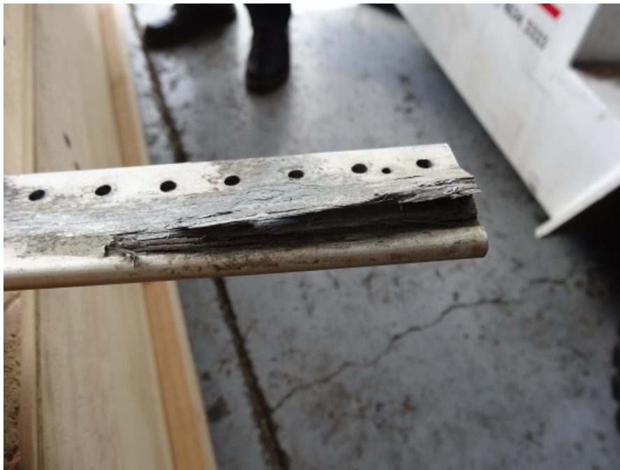
Cessna 100 series wing spar corrosion damage
