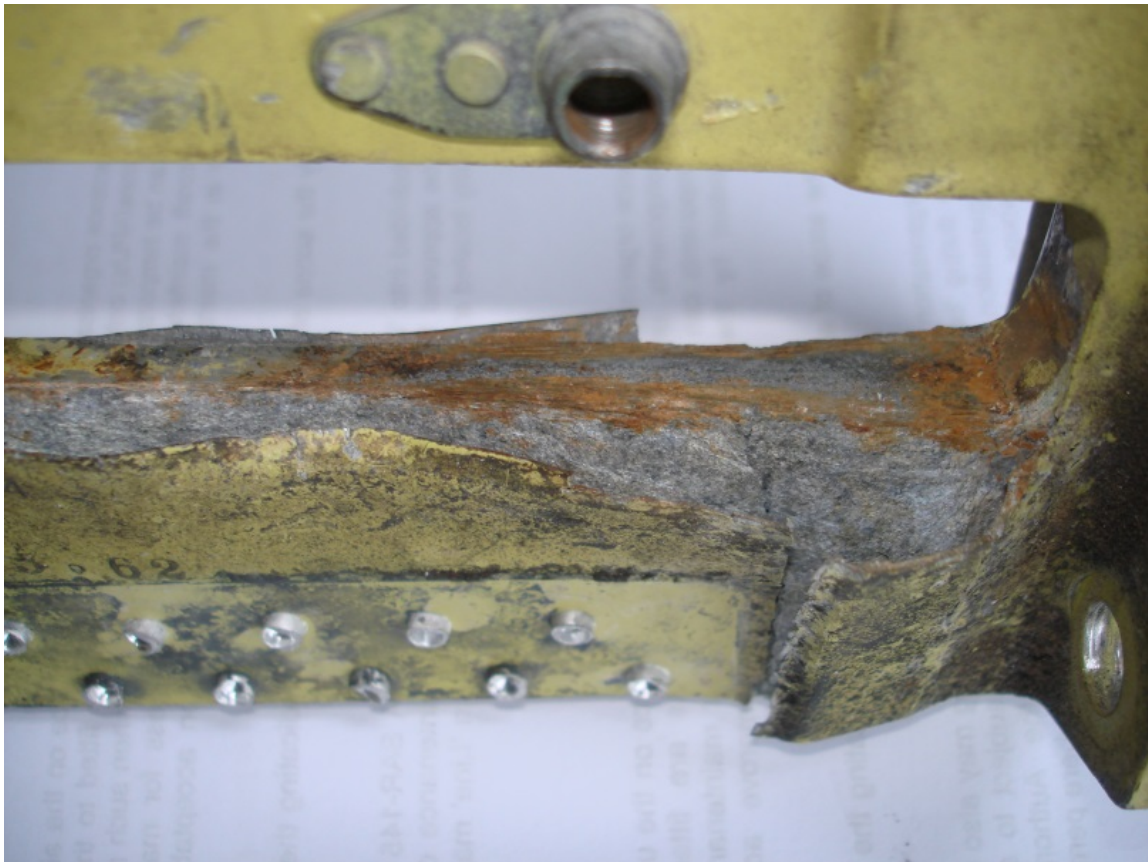
Cessna 100 series undercarriage bracket damage
