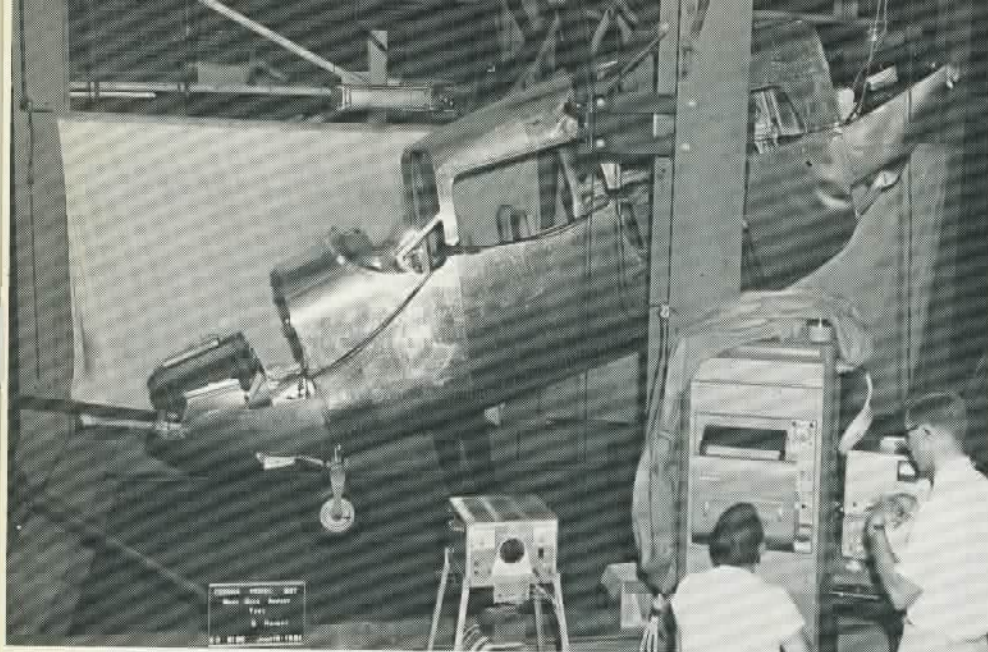
The picture isn't out of focus: Piper engineers are shaking the daylight out of an engine mount to measure how much vibration it can survive.
