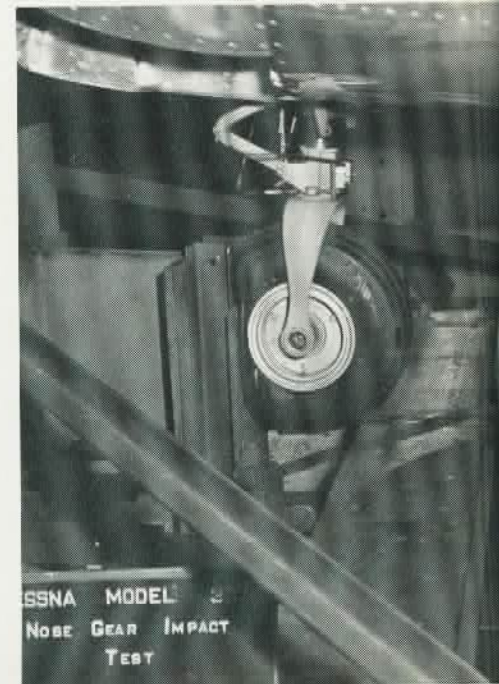
Engineers hammer a Skymaster's gear savagely during drop tests, seeking to measure exactly how much force it will take to cause structural failure.
