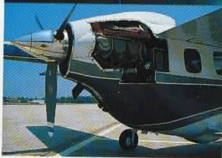
A peek under the jam-packed rear cowling confirms that the pusher engine is still a bear to work on.
