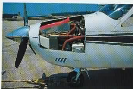
A Continental 310-hp engine is shoe-horned into the nose of this unique aircraft.
