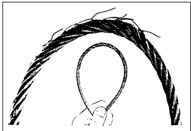
FIGURE 7-16. Cable inspection technique.
